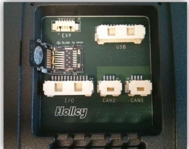
Figure 3. Insert micro-SD card
