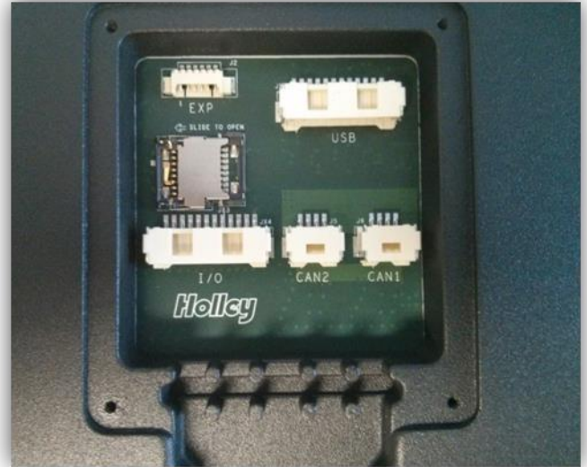
Figure 1. Slide door to the left to unlock
